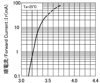
順電圧/Forward Voltage:  $V_F$  (V)
